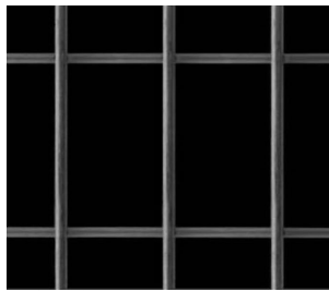
McNICHOLS® Wire Mesh Rectangular, Carbon Steel, Cold Rolled, Welded - Trimmed, 4" x 2" Mesh (Rectangular), 3.7500" x 1.7500" Opening (Rectangular), 0.2500" Thick (2-3/4 Gauge) Wire Diameter: 50% Open Area ITEM: 3642250141
