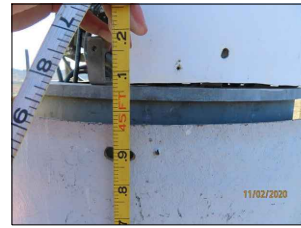
TOP OF SPRINT SHROUD CANISTER CONFIRMATION @ 45'-1"
