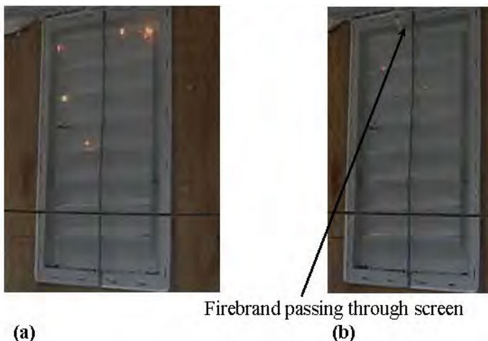
Figure 8 Images of the steel screen (3 mm) located behind the gable vent. Panel (b) shows a firebrand penetrating the screen after burning to a small enough size (see arrow).
