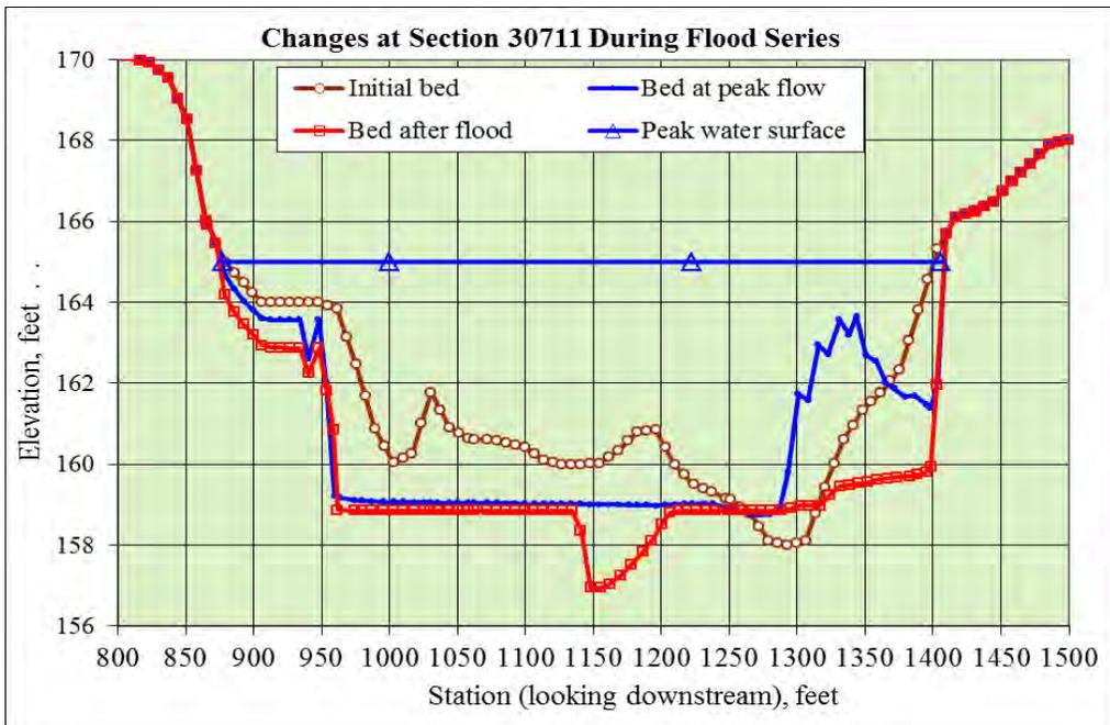
Figure 18. Simulated cross-sectional changes during flood series at channel station 30711
