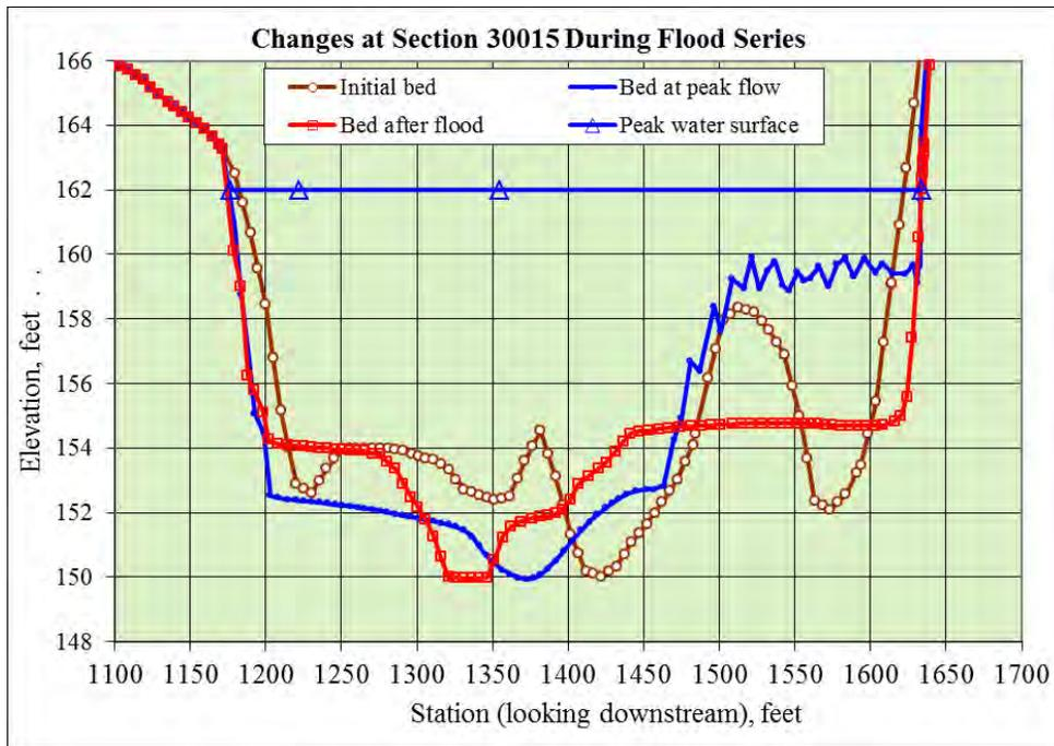
Figure 15. Simulated cross-sectional changes during flood series at channel station 30015
