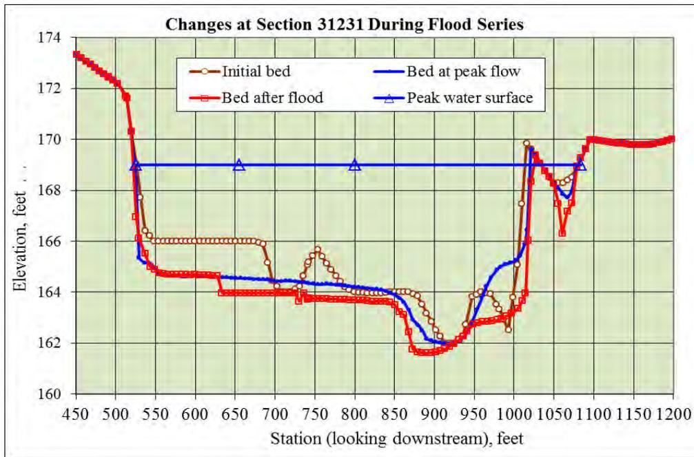
Figure 22. Simulated cross-sectional changes during flood series at channel station 31231
