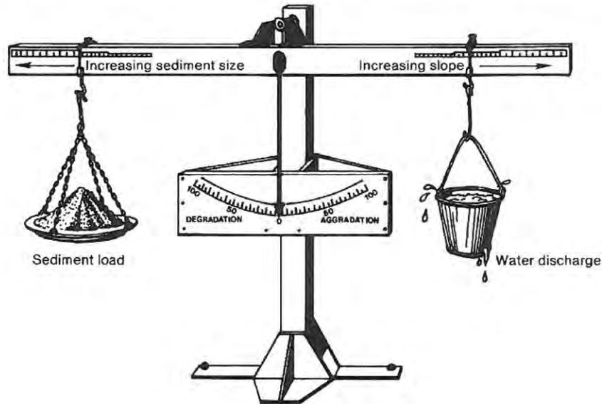
Figure 2. Stable channel balance (after Lane, 1955)
