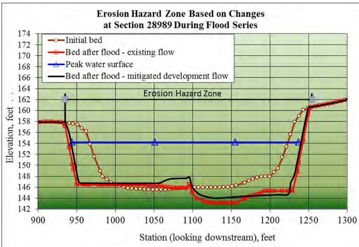
Figure 36. Erosion hazard zone based on the final cross-section profiles simulated using the existing flow and the mitigated development flow at channel station 28989
