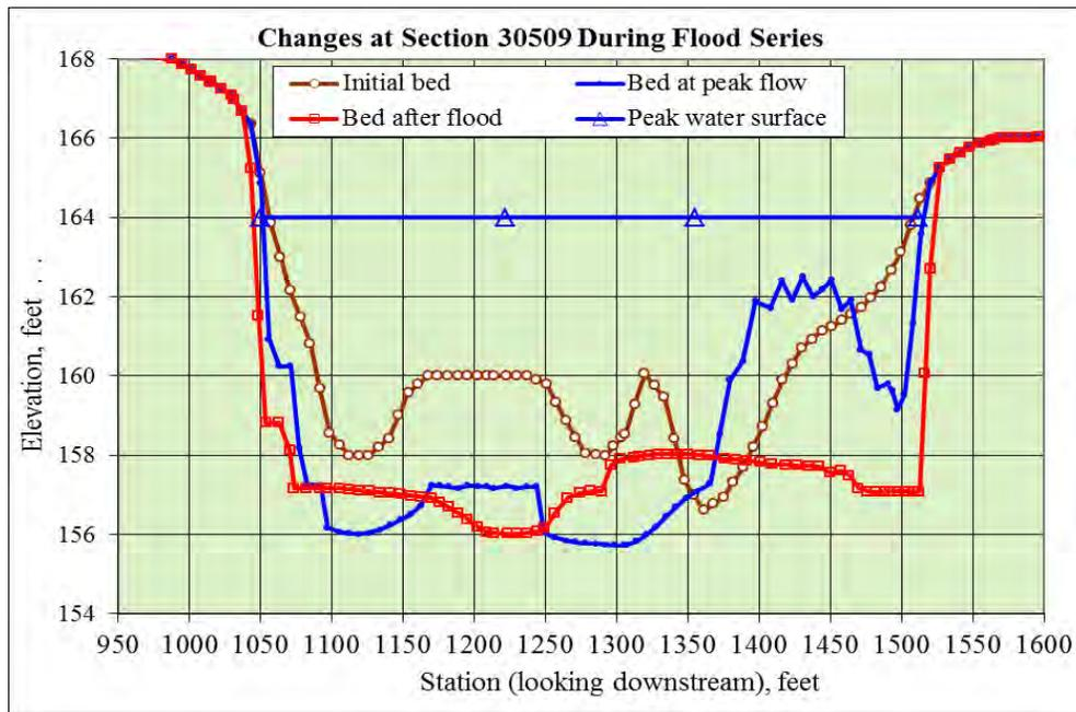
Figure 16. Simulated cross-sectional changes during flood series at channel station 30509
