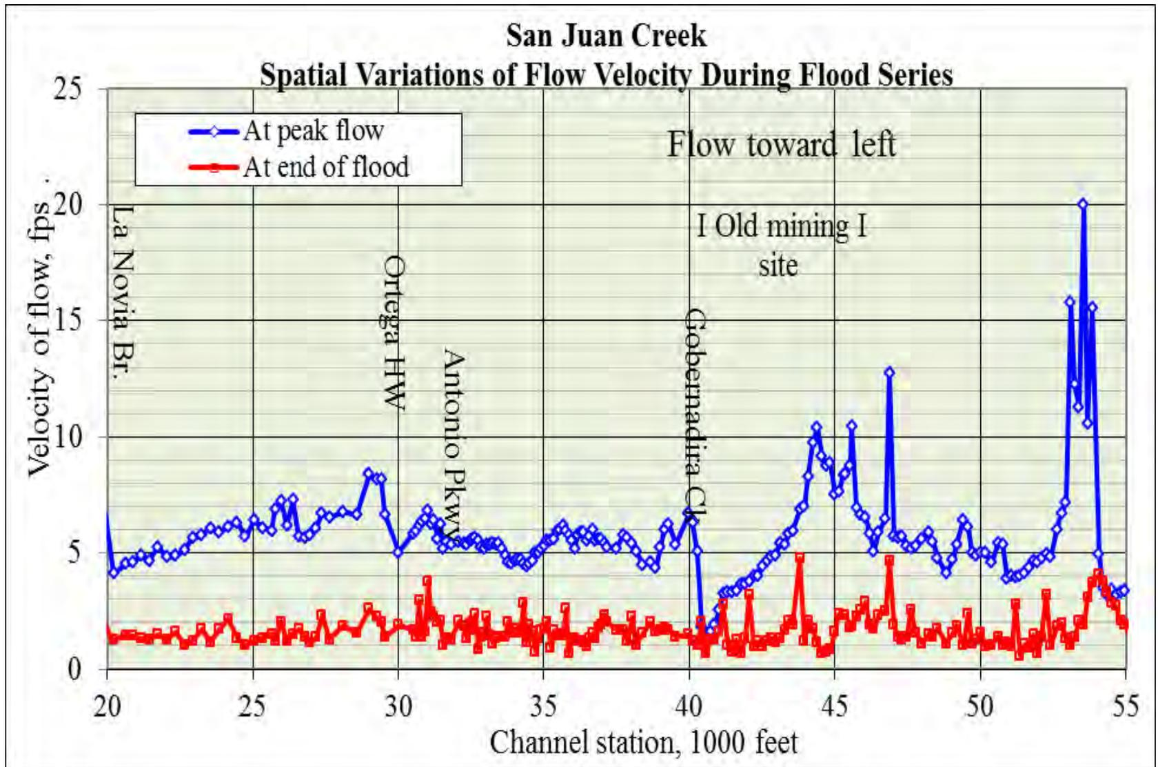
Figure 8. Time and spatial variations of flow velocity during 25-yr flood along river channel
