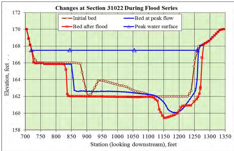
Figure 20. Simulated cross-sectional changes during flood series at channel station 31022
