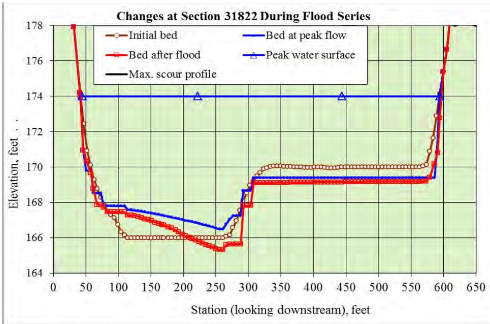
Figure 27. Simulated cross-sectional changes during flood series at channel station 31822
