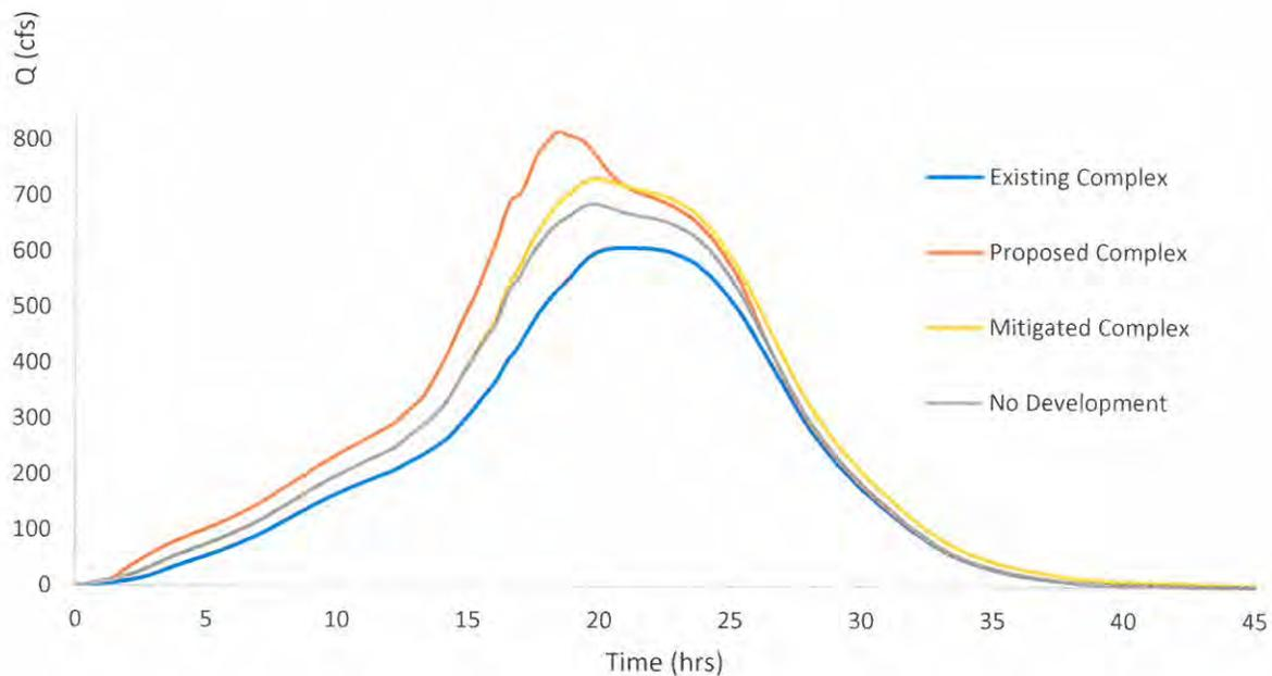
**Figure 1 – 2-year Sensitivity Analysis at Downstream RMV Boundary (Node 137) Removing All Proposed RMV Development**
