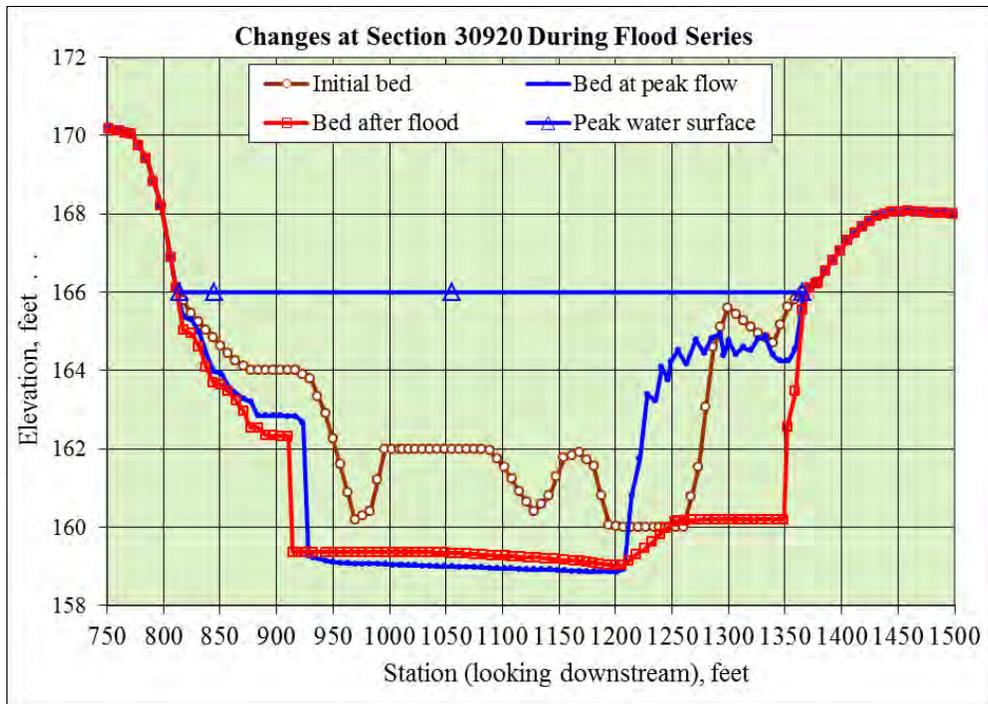
Figure 19. Simulated cross-sectional changes during flood series at channel station 30920
