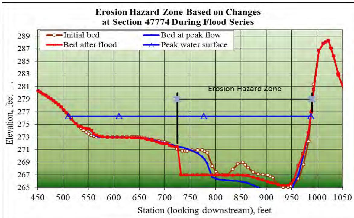
Figure 33. Erosion hazard boundary based on simulated cross-sectional changes during flood series at channel station 47774. At this wide channel section, the erosion hazard zone is smaller than the channel width.
