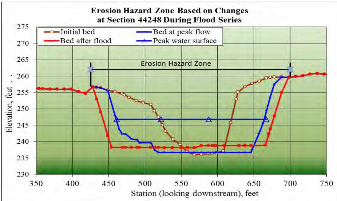
Figure 32. Erosion hazard boundary based on simulated cross-sectional changes during flood series at channel station 44248. This channel station is located at the upstream entrance to the old mining site. It is predicted to undergo major increase in width. The erosion hazard zone is much wider than the existing channel width..
