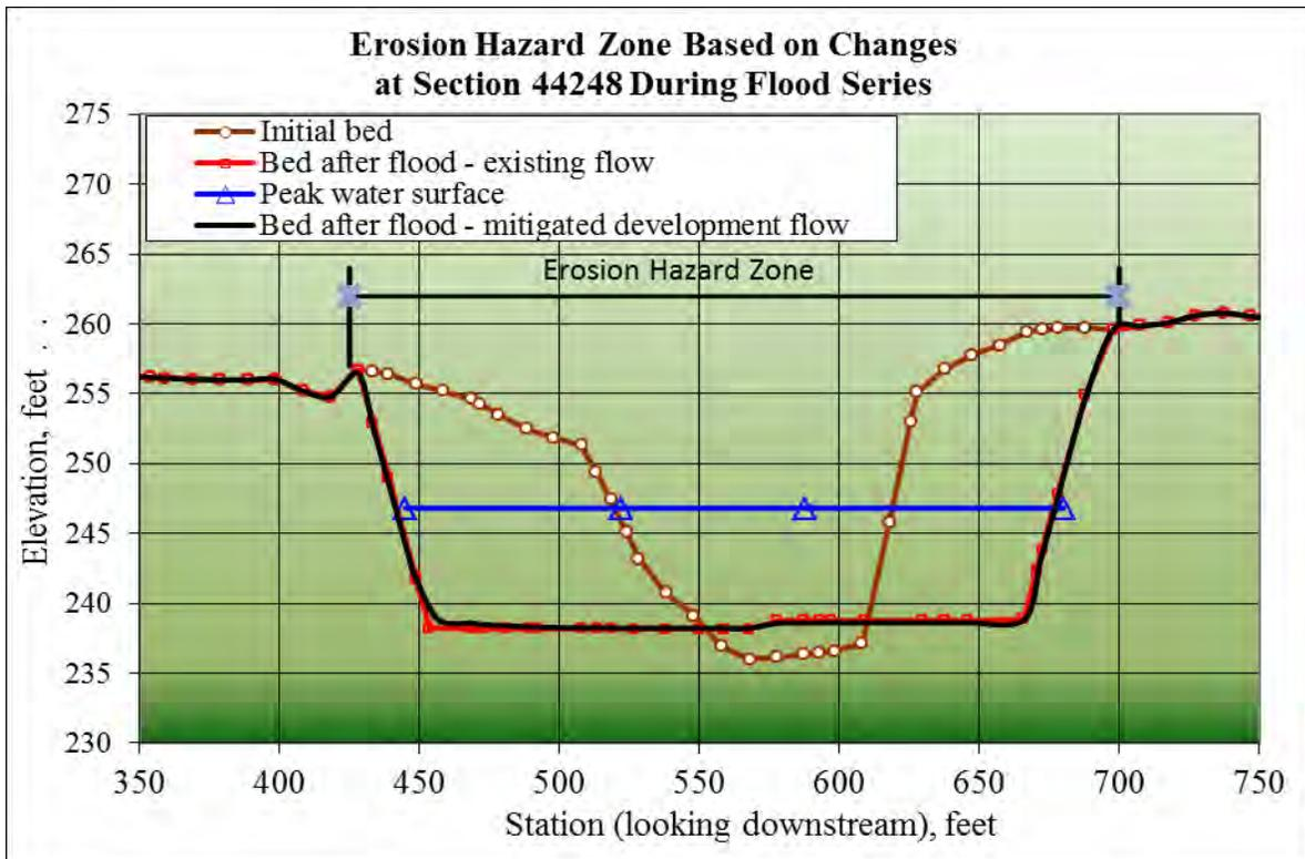
Figure 39. Erosion hazard zone based on the final cross-section profiles simulated using the existing flow and the mitigated development flow at channel station 44248
