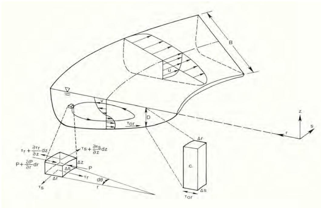
Figure 3. Components of flow through a curved channel
