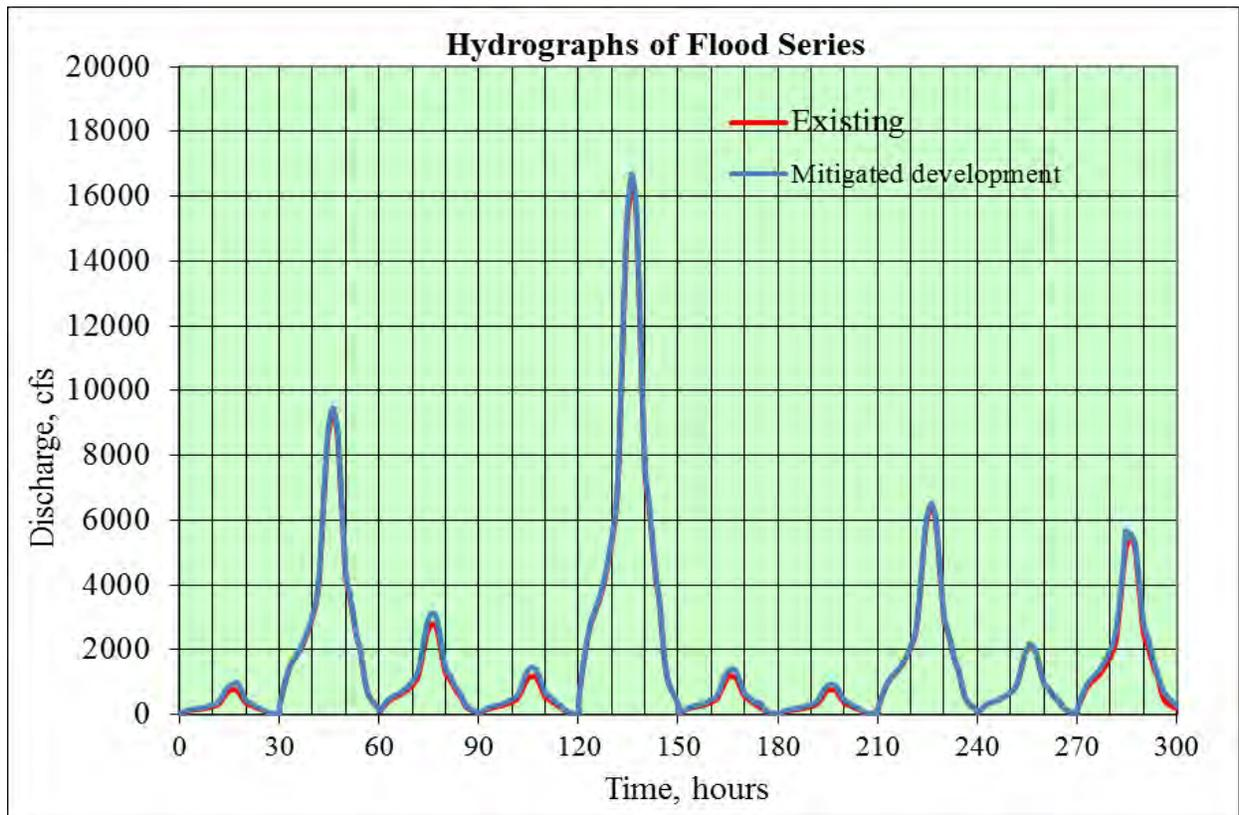
Figure 7B. Hydrograph of the flood series for existing and mitigated development conditions
