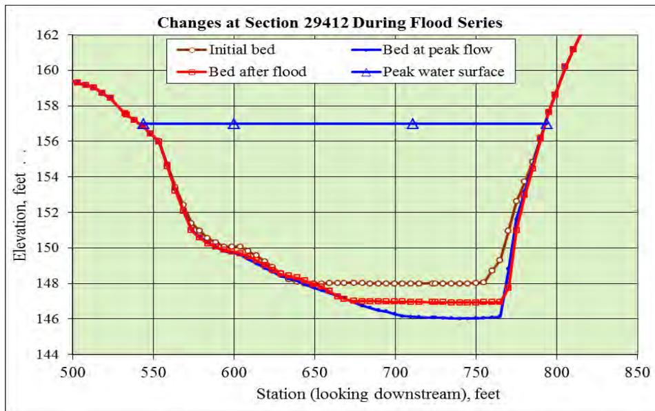
Figure 13. Simulated cross-sectional changes during flood series at channel station 29412
