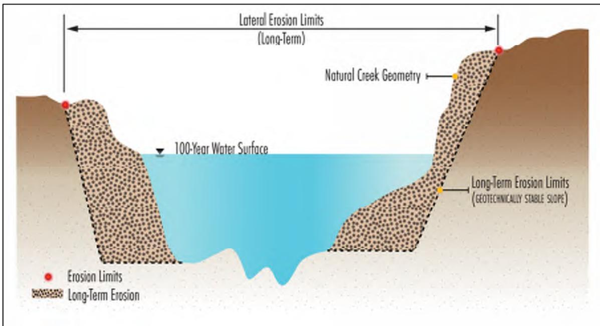
**Figure 1 - Typical Channel Section Lateral Erosion Limits**
