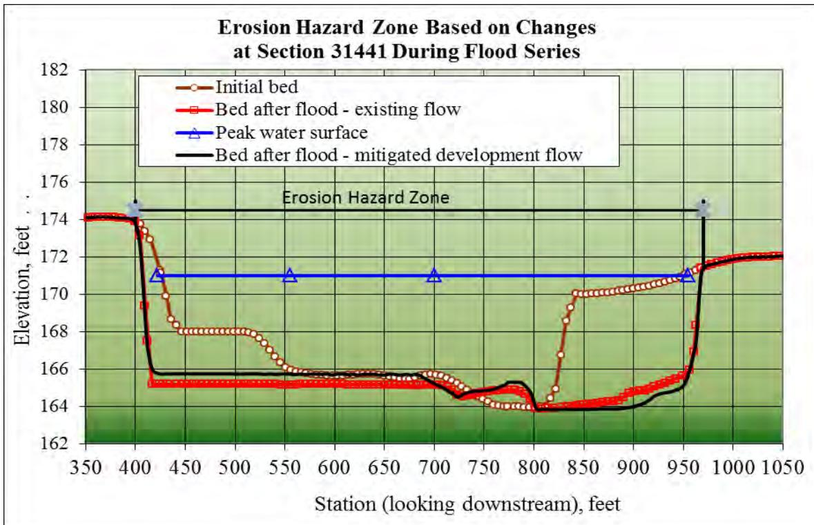
Figure 37. Erosion hazard zone based on the final cross-section profiles simulated using the existing flow and the mitigated development flow at channel station 31441
