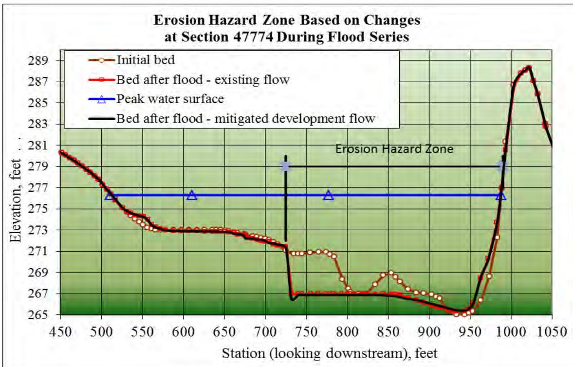
Figure 40. Erosion hazard zone based on the final cross-section profiles simulated using the existing flow and the mitigated development flow at channel station 47774
