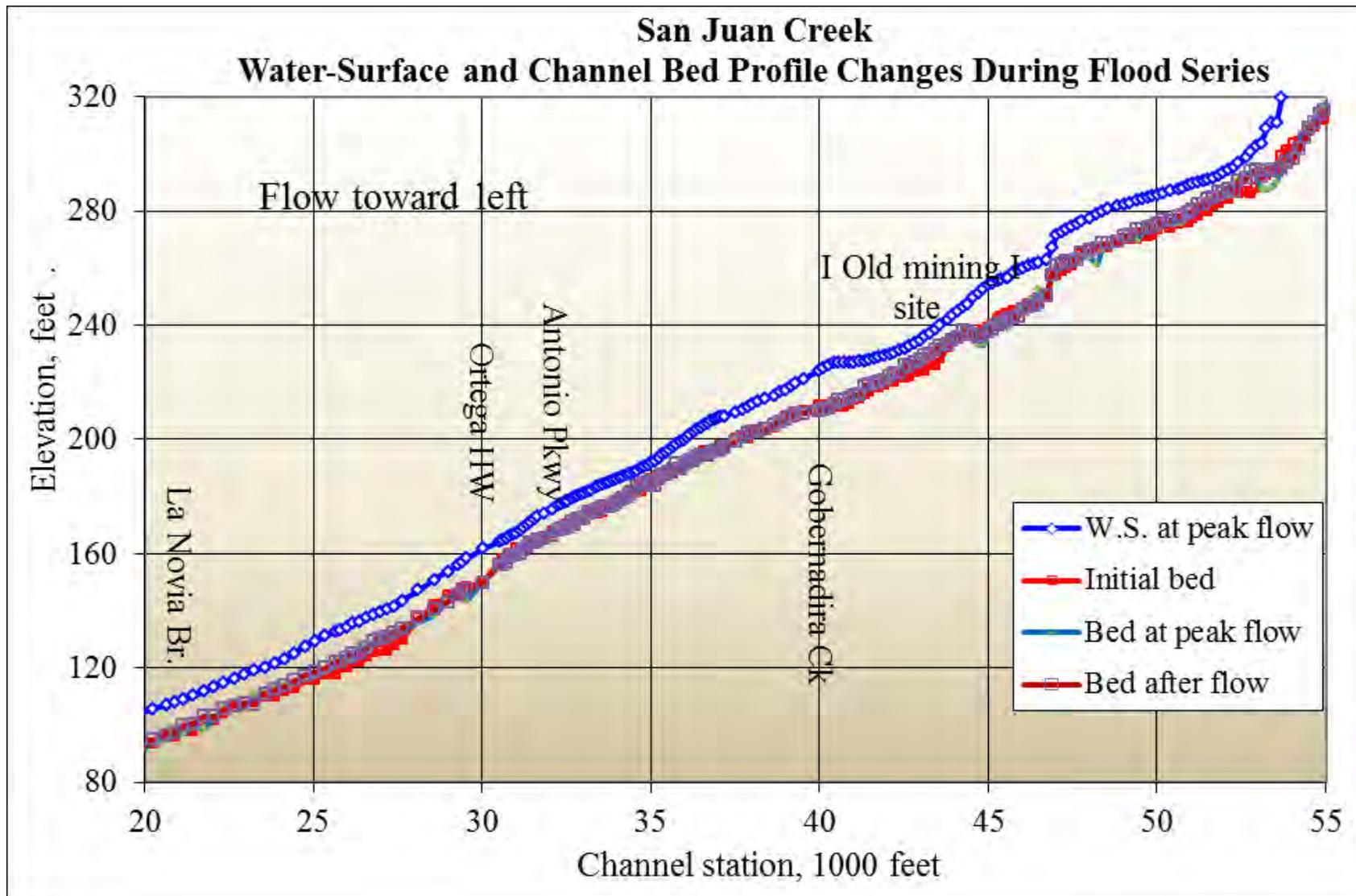
Figure 11. Water-surface and channel bed profile changes during flood series
