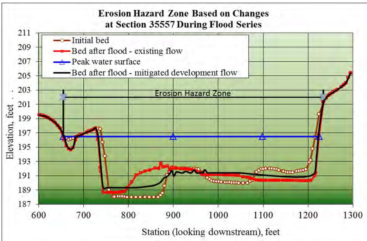
Figure 38. Erosion hazard zone based on the final cross-section profiles simulated using the existing flow and the mitigated development flow at channel station 35557
