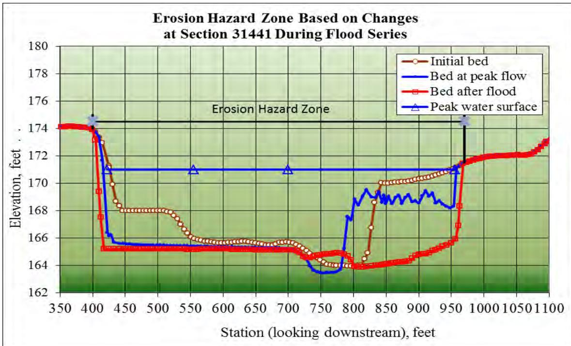
Figure 30. Erosion hazard boundary based on simulated cross-sectional changes during flood series at channel station 31441. The erosion hazard zone at this channel station is wider than the existing channel. This section is predicted to undergo major lateral migration toward the right bank. \*
