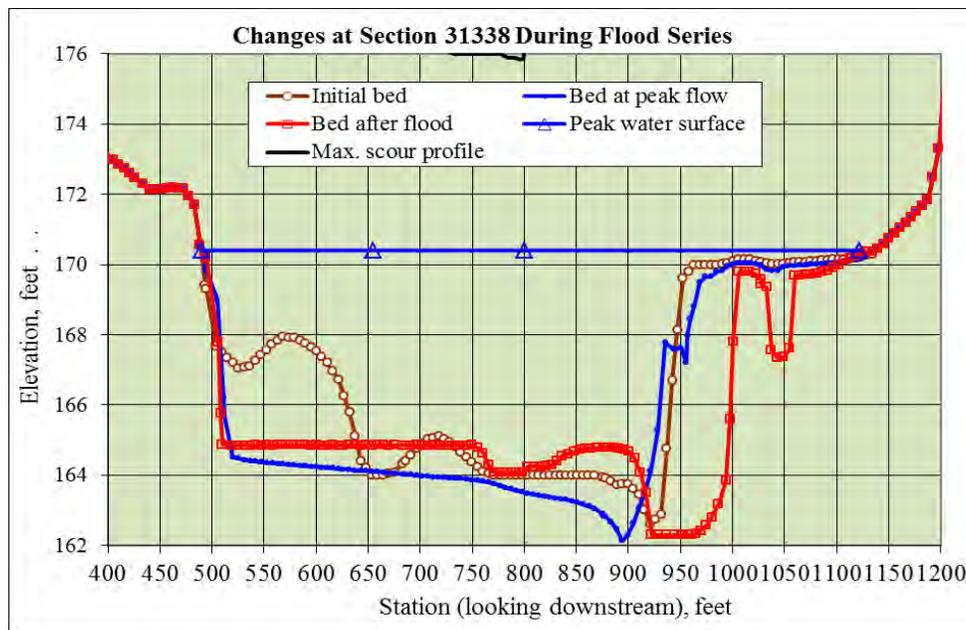
Figure 23. Simulated cross-sectional changes during flood series at channel station 31338
