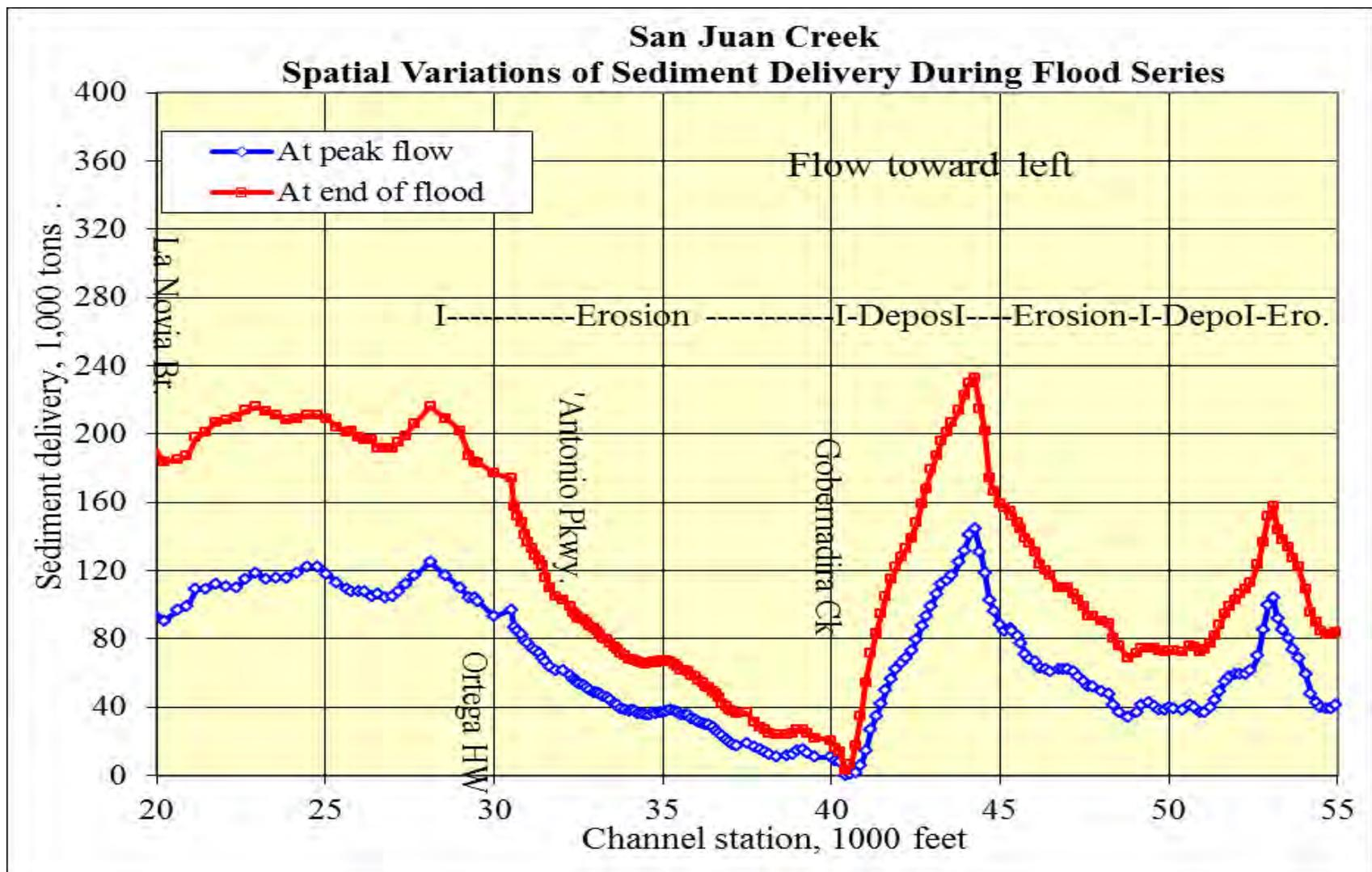
Figure 10. Time and spatial variations of sediment delivery during the flood series
