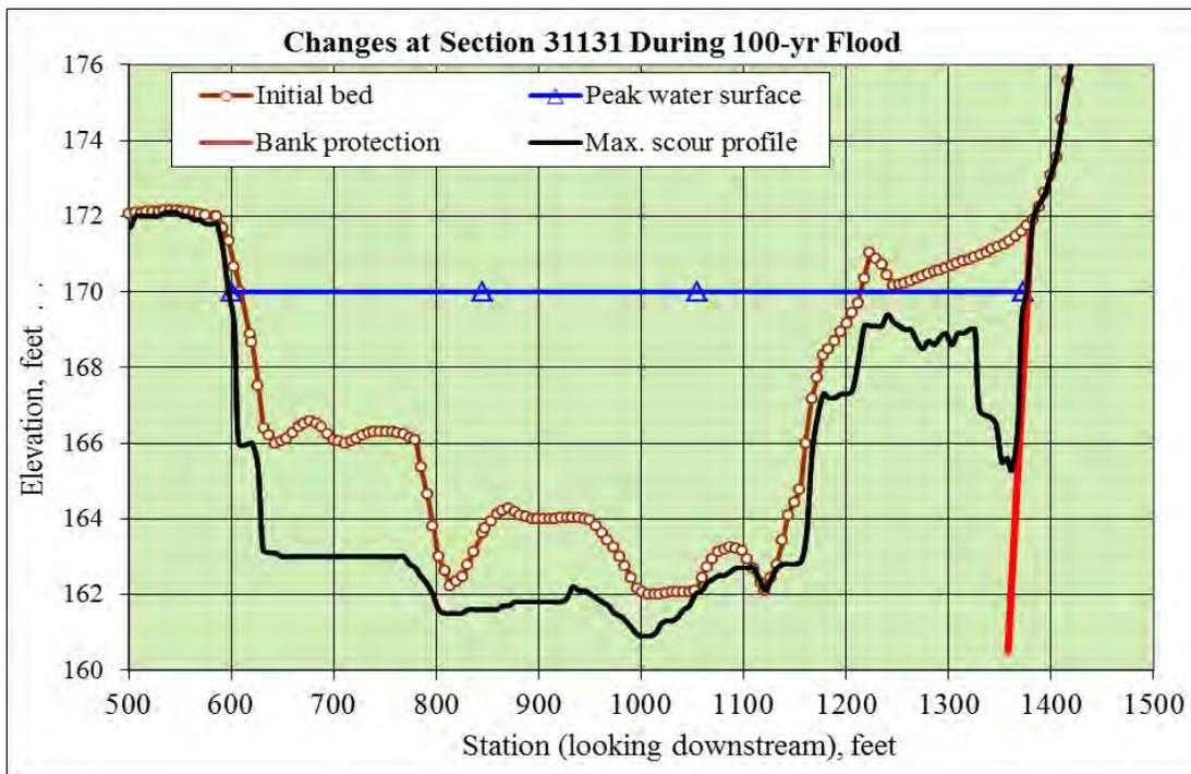
Figure 37. Design of bank protection in consideration of potential channel bed scour at bank toe
