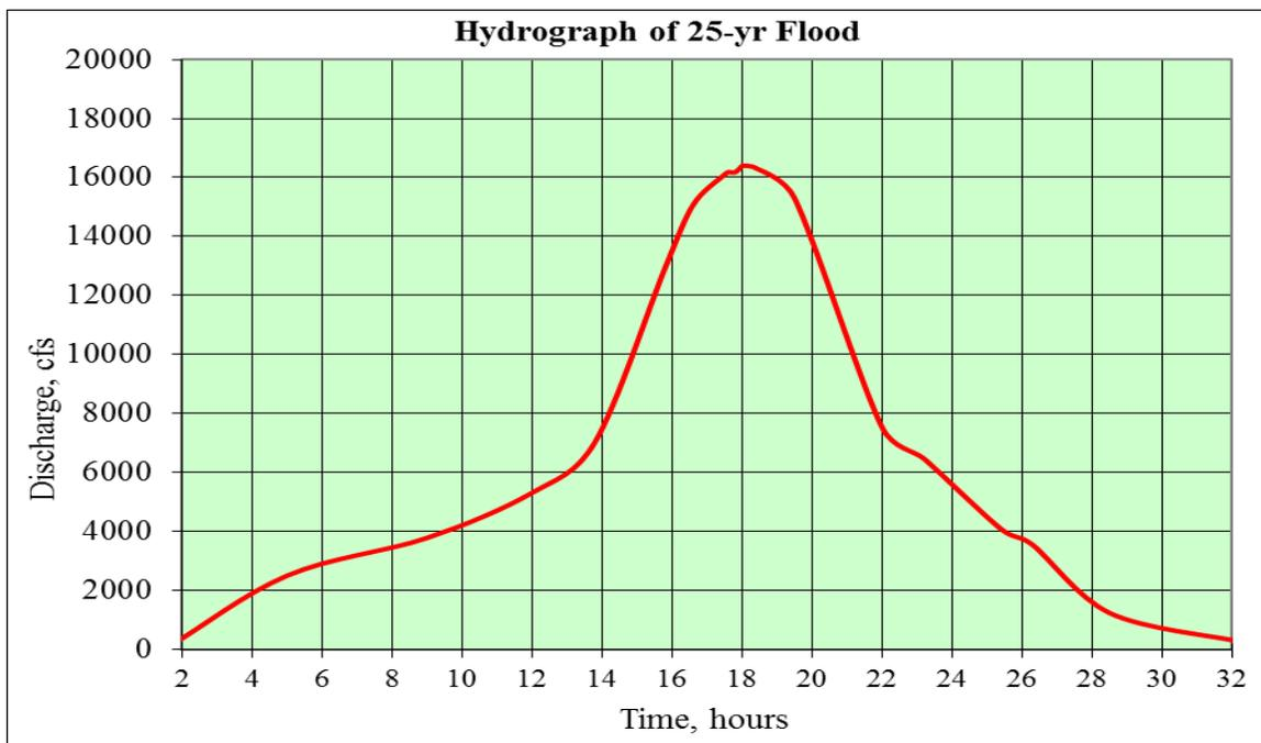
Figure 6. Hydrograph of the 25-yr flood
