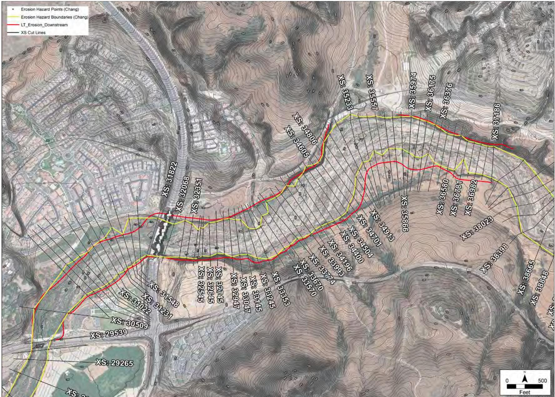
Figure 34. Erosion hazard zone for downstream area
