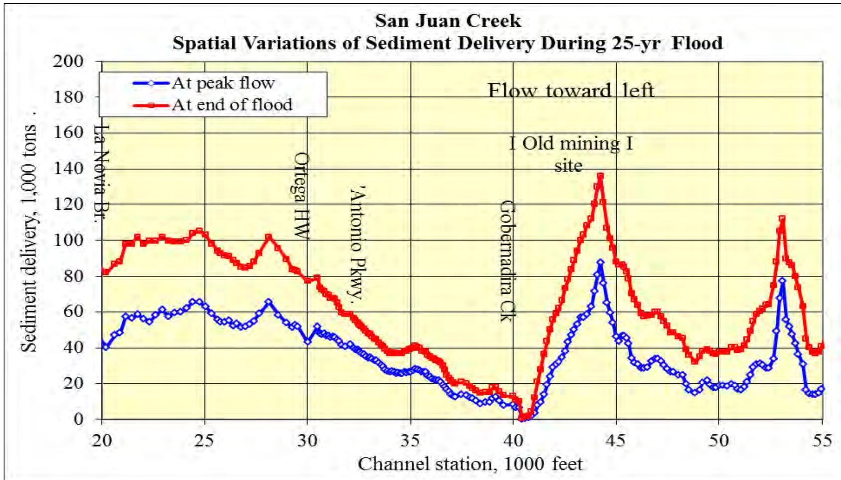
Figure 9. Time and spatial variations of sediment delivery during the 25-yr flood
