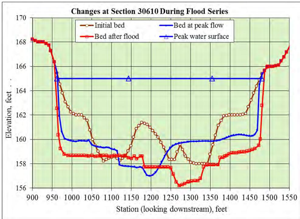
Figure 17. Simulated cross-sectional changes during flood series at channel station 30610
