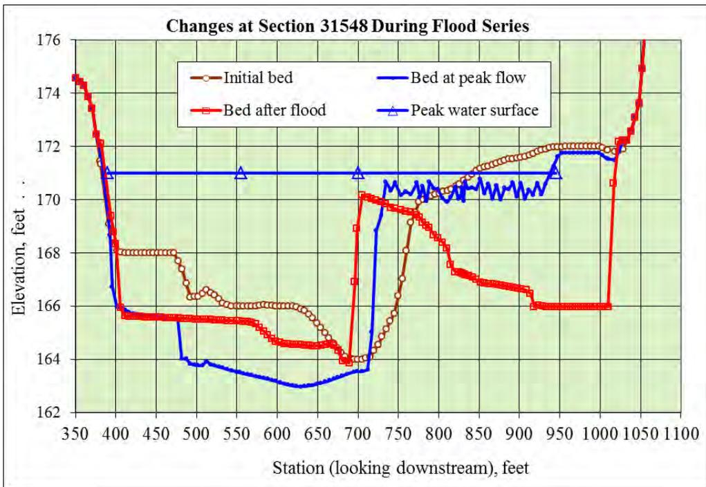
Figure 25. Simulated cross-sectional changes during flood series at channel station 31548
