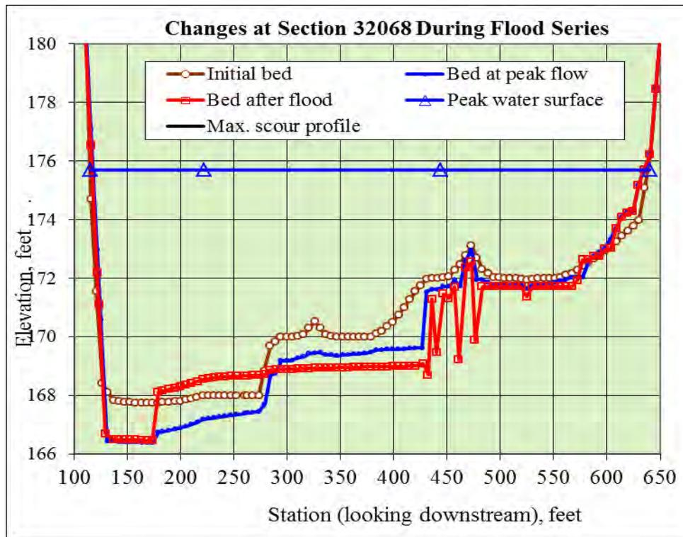
Figure 28. Simulated cross-sectional changes during flood series at channel station 32068
