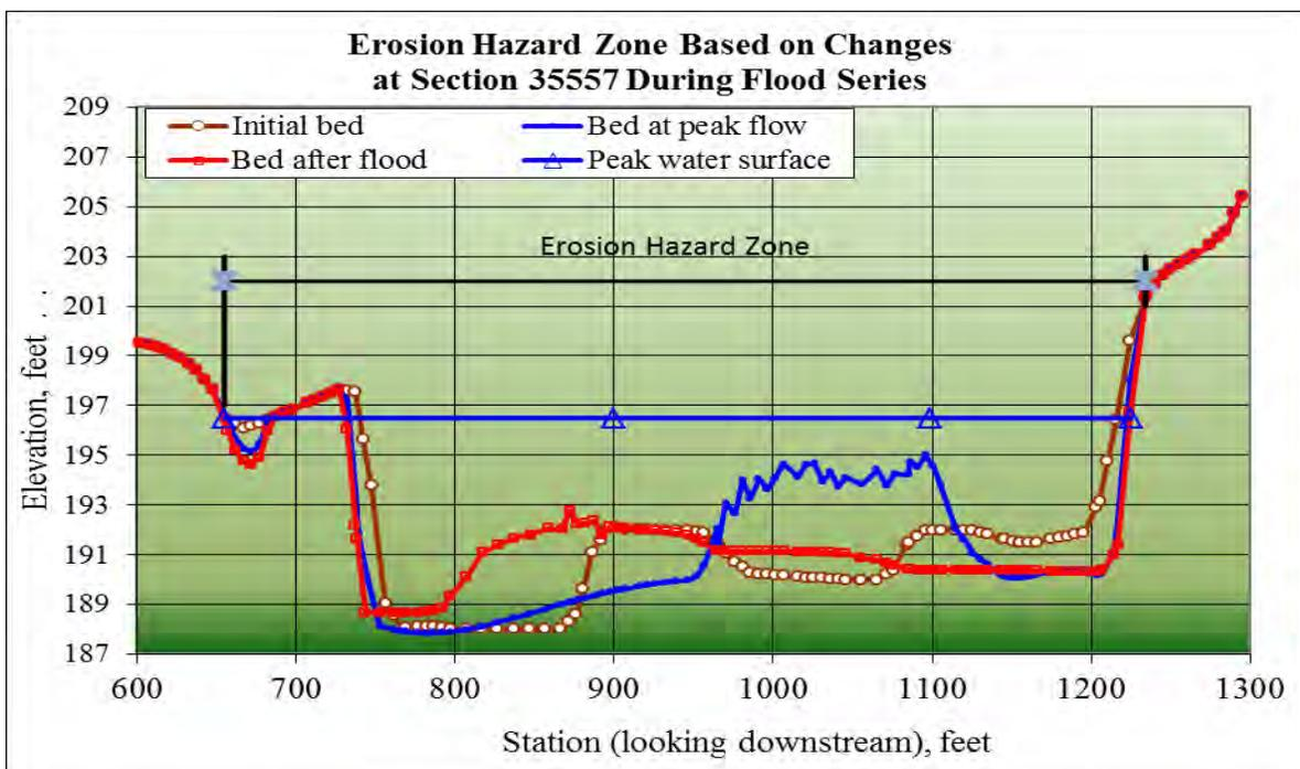
Figure 31. Erosion hazard boundary based on simulated cross-sectional changes during flood series at channel station 35557. The erosion hazard zone at this channel station is the same as the existing channel width.
