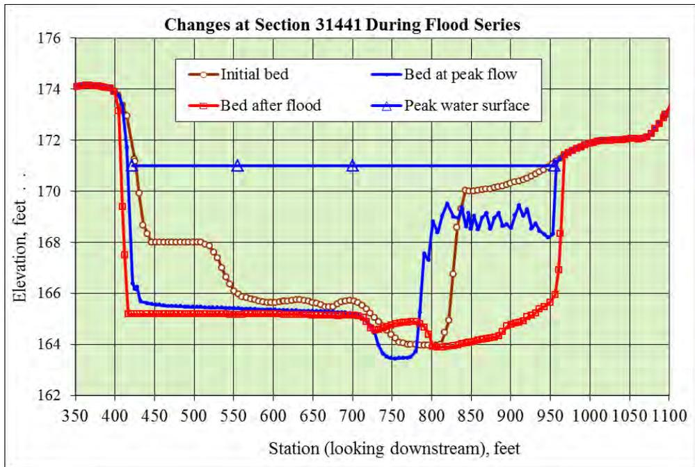
Figure 24. Simulated cross-sectional changes during flood series at channel station 31441
