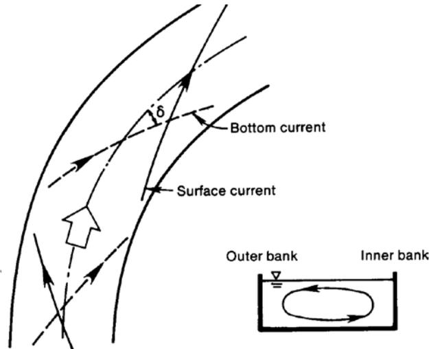
Figure 4. Surface and bottom currents in a curved channel
