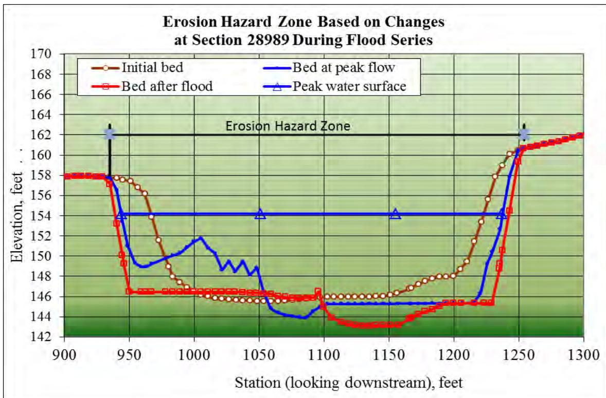
Figure 29. Erosion hazard boundary based on simulated cross-sectional changes during flood series at channel station 28989. The erosion hazard zone at this channel station is wider than the existing channel width. This section is predicted to widen as both banks retreat during the flood series.
