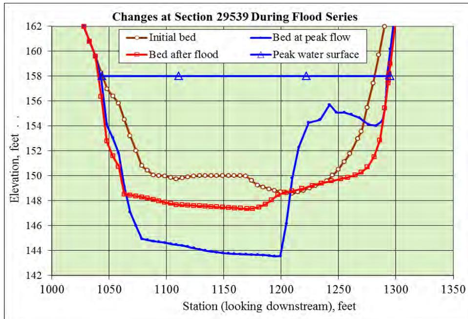
Figure 14. Simulated cross-sectional changes during flood series at channel station 29539
