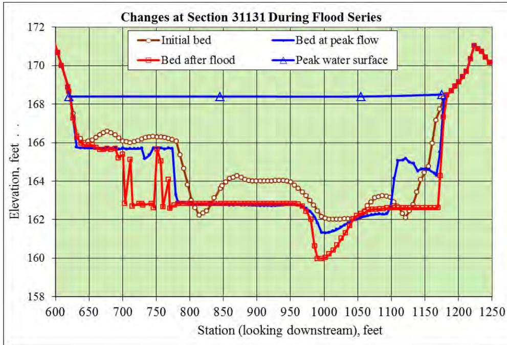
Figure 21. Simulated cross-sectional changes during flood series at channel station 31131
