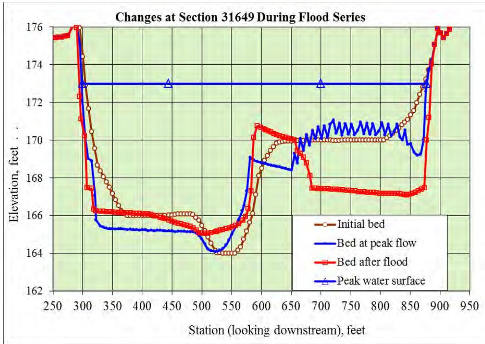
Figure 26. Simulated cross-sectional changes during flood series at channel station 31649
