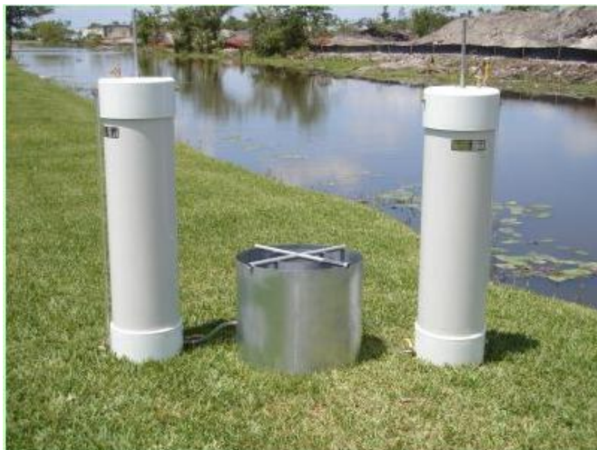
Figure VII.10. Double Ring Infiltrometer Set-up with Mariotte Tubes
