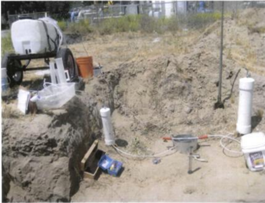
Figure VII.11. Double Ring Infiltrrometer Set-up for Test at Basin Surface Elevation
